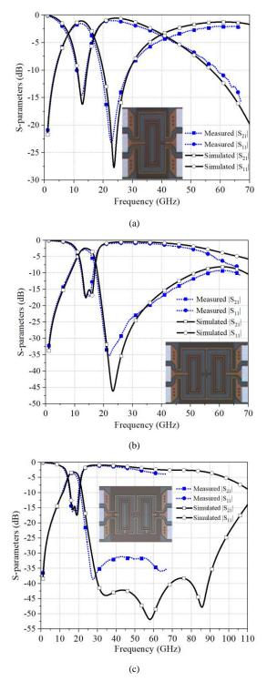
Fig. 21. Measured S-parameters of all three designs, (a) 1<sup>st</sup>-order BPF, (b) 2<sup>nd</sup>-order BPF, (c) modified 2<sup>nd</sup>-order BPF with improved out-of-band suppression.
