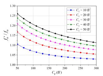
Fig. 18. The frequency ratio of  $f'_o/f_o$  against  $C_p$  when  $C_1$  varies from 10 fF to 50 fF.
