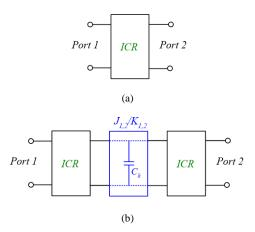
Fig. 11. Configuration of (a) a conventional 1<sup>st</sup>-order BPF; (b) a conventional 2<sup>nd</sup>-order BPF. Note: ICR stands for inverting-coupled resonator.
