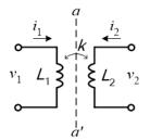
Fig. 5. A two-port network comprising two inductors including mutual coupling.
