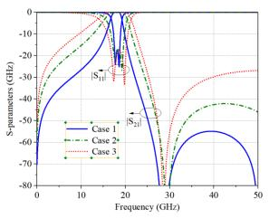
Fig. 17. S-parameters of three  $2^{nd}$ -order BPFs using MICR with different bandwidths.
