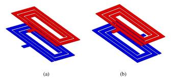
Fig. 2. Two types of resonators using coupled inductors: (a) non-inverting coupled type; (b) inverting coupled type.
