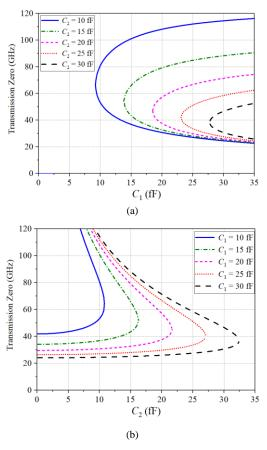
Fig. 10. The values of transmission zeros (a) varying against  $C_1$  when  $C_2$  is fixed; (b) varying against  $C_2$  when  $C_1$  is fixed.
