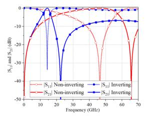
Fig. 6. Calculated *S*-parameters of two filters using inverting- and non-inverting- coupled structures. Related parameter values are:  $L_1 = 1000$  pH,  $C_1 = 30$  fF,  $C_2 = 10$  fF, and k = -0.8 (inverting coupling) and 0.8 (non-inverting coupling).
