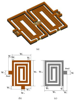
Fig. 19. Layout of the modified 2<sup>nd</sup>-order BPF: (a) 3-D view of the modified 2<sup>nd</sup>-order BPF, (b) upper spiral layer; and (c) lower spiral layer. Note:  $W_1 = 6 \mu m$ ,  $W_2 = 74 \mu m$ ,  $W_3 = 4 \mu m$ ,  $W_4 = 180 \mu m$ ,  $W_5 = 12 \mu m$ ,  $W_6 = 12 \mu m$ ,  $W_7 = 6 \mu m$ ,  $W_8 = 74 \mu m$ ,  $W_9 = 4 \mu m$ ,  $W_{10} = 180 \mu m$ ,  $W_{11} = 12 \mu m$ ,  $W_{12} = 12 \mu m$ ,  $W_{13} = 12 \mu m$  and  $W_{14} = 12 \mu m$ .
