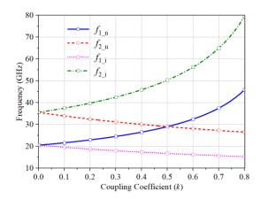
Fig. 7. Resonant mode distribution of  $f_{1_n}$ ,  $f_{2_n}$ ,  $f_{1_i}$  and  $f_{2_i}$  against k. Related parameter values are:  $L_1 = 1000$  pH,  $C_1 = 20$  fF,  $C_2 = 20$  fF.
