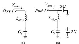
Fig. 4. Even- and odd-mode analysis of the *LC*-equivalent circuit: (a) even-mode, (b) odd-mode.
