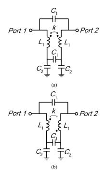
Fig. 3. Simplified *LC*-equivalent circuit models for the resonators in Fig. 2: (a) with non-inverting coupled one; (b) with inverting coupled one.
