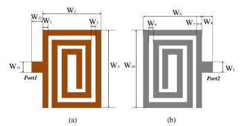
Fig. 14. Layout of the 1<sup>st</sup>-order BPF: (a) upper layer spiral, and (b) lower layer spiral. Note:  $W_1 = 6 \ \mu m$ ,  $W_2 = 74 \ \mu m$ ,  $W_3 = 4 \ \mu m$ ,  $W_4 = 190 \ \mu m$ ,  $W_5 = 12 \ \mu m$ ,  $W_6 = 12 \ \mu m$ ,  $W_7 = 6 \ \mu m$ ,  $W_8 = 74 \ \mu m$ ,  $W_9 = 4 \ \mu m$ ,  $W_{10} = 190 \ \mu m$ ,  $W_{11} = 12 \ \mu m$ , and  $W_{12} = 12 \ \mu m$ .
