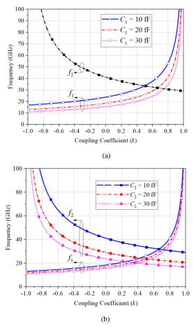
Fig. 8. The values of resonant poles against coupling coefficient k when different values of  $C_1$  and  $C_2$  are chosen: (a)  $C_1$  is varied from 10 to 30 fF, (b)  $C_2$  is varied from 10 to 30 fF.
