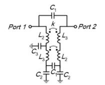
Fig. 15. Simplified *LC*-equivalent circuit of the modified inverting-coupled resonator.
