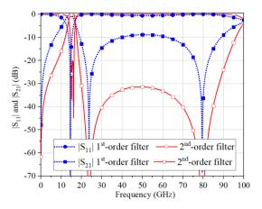
Fig. 12. S-parameters of the designed BPFs using inverting-coupled structure.
