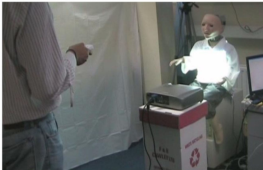
Figure 5.3: illustrates the experimental layout of the human-humanoid interaction experiment. A participant was holding a Wii Remote to perform a gesture pattern. The trajectories produced was projected onto the body of KASPAR2 using a projector.
