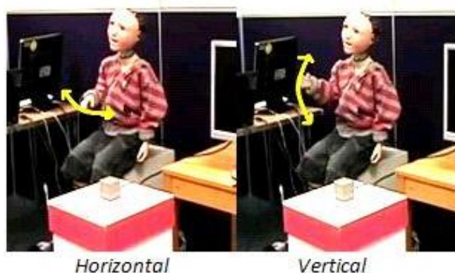
Figure 4.1: Illustration for KASPAR2's arm movements in horizontal and vertical direction.
