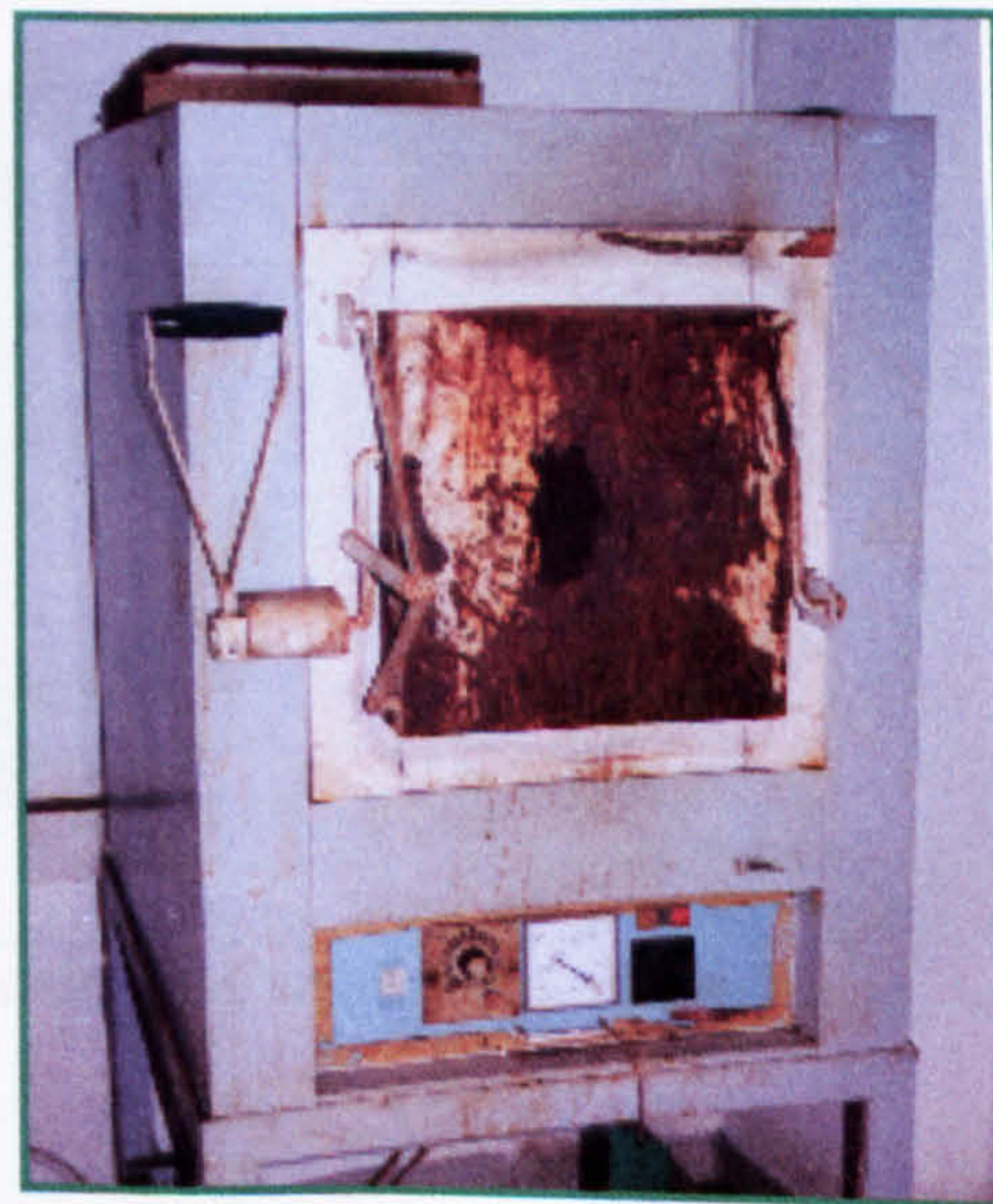
Figure B.7 Electric furnace used for the expansion of retainment ring
