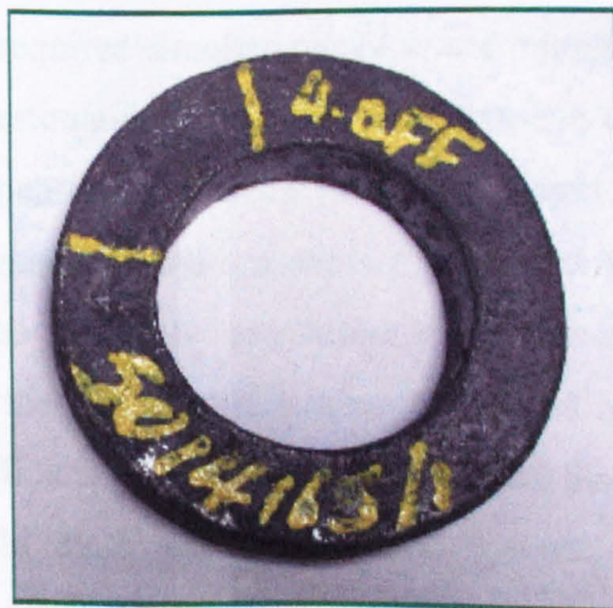
Figure A.6 Forged ring of Maraging G125
