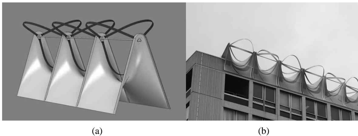
Figure 2.18: Crossflow wind turbine: (a) concept; (b) architectural integration with ridge [79].
