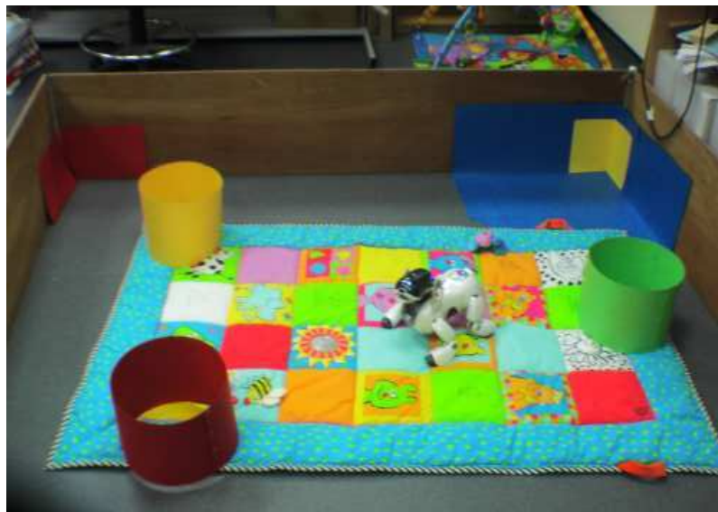
Figure 5.3: The experimental setup. An AIBO robot was placed on a children's play mat in a wooden arena where several toys and large objects can be perceived.
