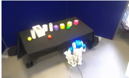
Figure 7.10: The more complex environment used in the second set of tests of the robot profiles. More objects that vary in shapes and sizes were placed on the table.
