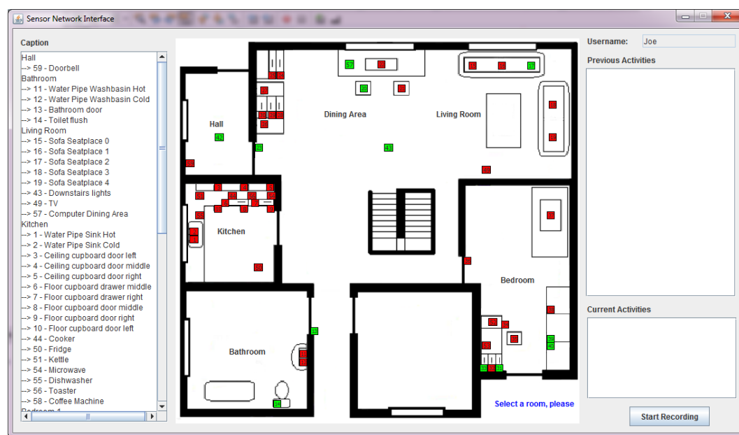
Figure 3.4: ARS Graphical Interface - Sensors installed around the Robot House
