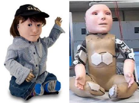
Fig. 1 The robot KASPAR. The figure on the right shows the 'undressed' version revealing the tactile skin patches
