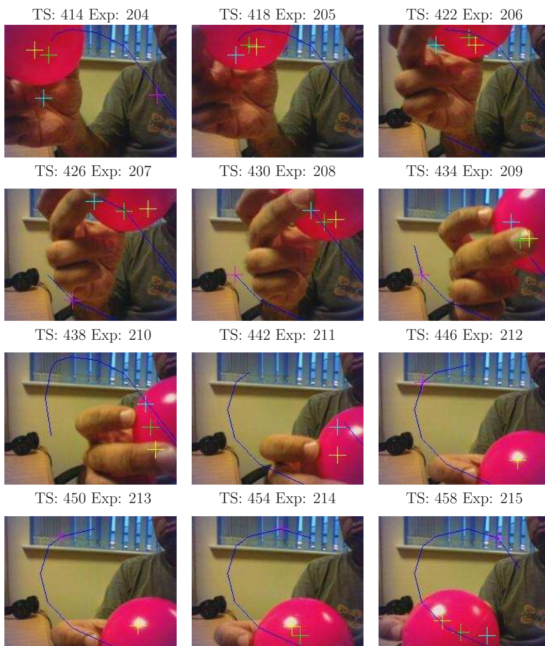
Figure 5.7: Series of 12 consecutive images from the Aibo camera showing ball path prediction using a sensorimotor experience space. The robot does not move its head in this sequence. Images are sequential left to right and top to bottom. The sequence lasts approx. 4 seconds (44 timesteps or 12 experiences) and is taken after 37 seconds of activity. The line shows the path prediction for 10 experiences ahead. The crosses are from various methods for ball detection, only one of these was actually used as sensory input. h = 40 , Q = 5 , Experience granularity G = 4 timesteps. One image shown per experience.
