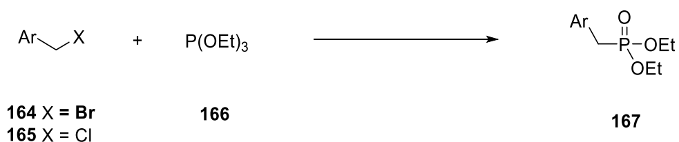
Scheme 2.4 Synthesis of benzylphosphonates
