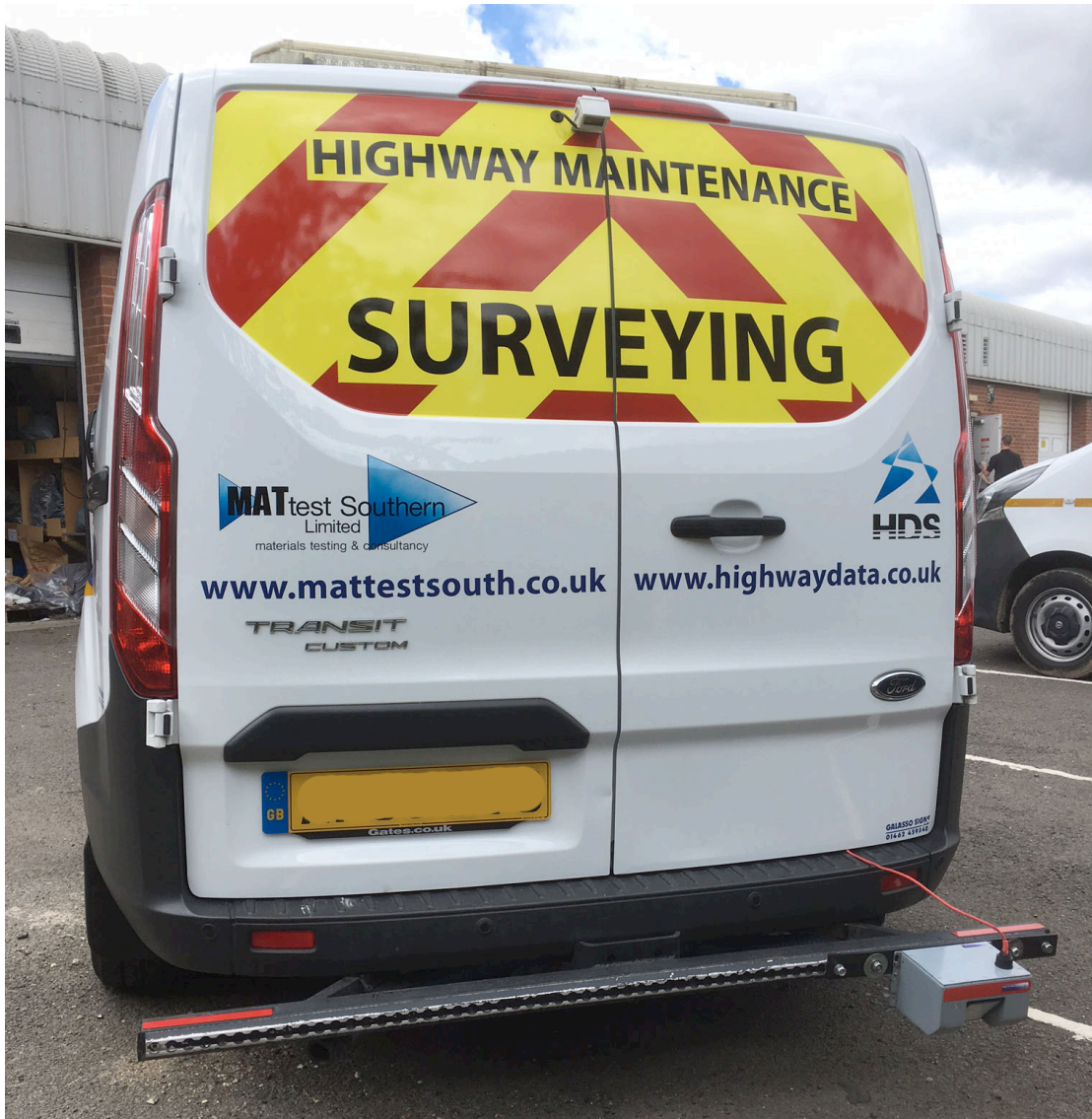
Figure 4-7 Test setup of LBRM device mounted on vehicle
