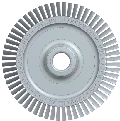
FIGURE 2: VIEW OF THE FULL BLADED DISC SYSTEM WITH UNDERPLATFORM DAMPERS.
