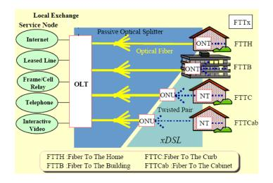
Figure 1-2 Fibre-to-the-x architectures [12]
