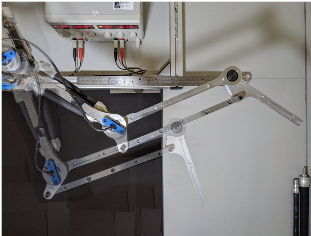
Fig. 1 Span-wise morphing structure in a fully extended position and retracted overlaid. Each pneumatic artificial muscle (PAM) antagonistic pair is visible actuating each respective joint.
