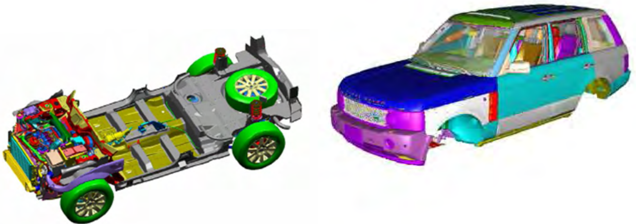
Figure 2.1.4 – CAD Models of a Vehicle Platform and Upper Body (source: RLE)
